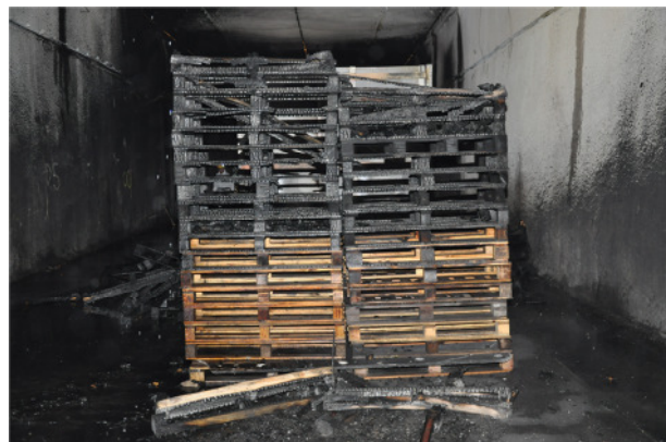
Fig. 16: Spread of fire to a further object at a distance of 5 m during a fire test without FFFS
