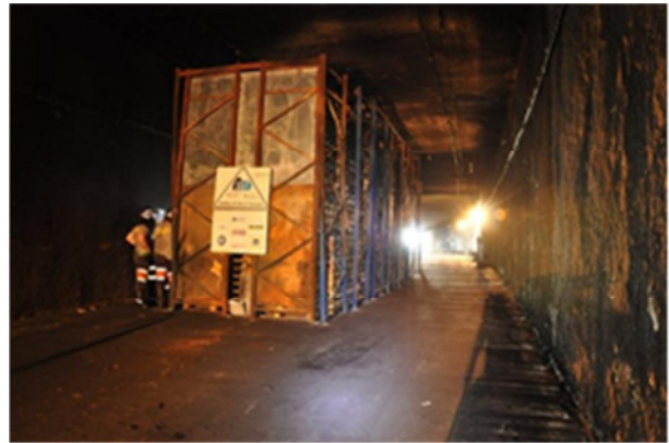
Fig.34: Typical truck fire load with chassis
