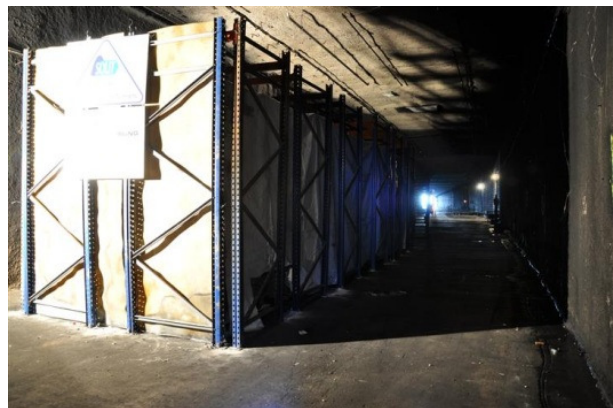
Fig. 35: Typical fire load without chassis to give a larger distance between the fire load and the tunnel roof
