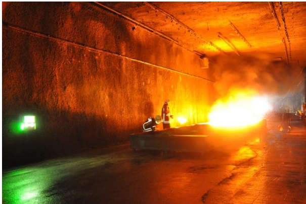
Figure 25: Ignition of the 60 MW pool
