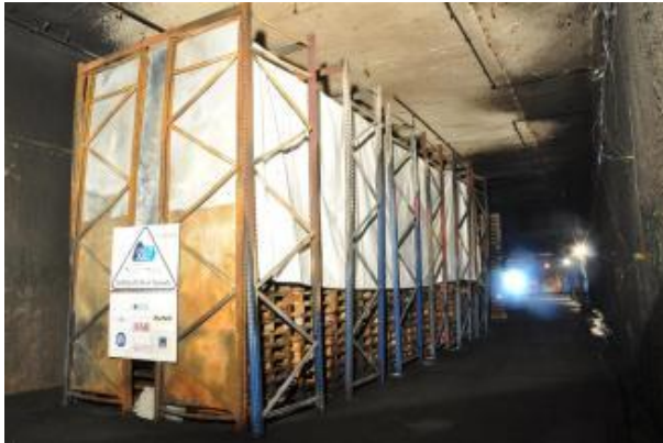
Figure 7: SOLIT Truck Fire Load with Cover
