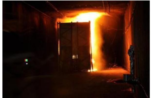
Figure 8: SOLIT Truck Fire Load shortly before activating the FFFS
