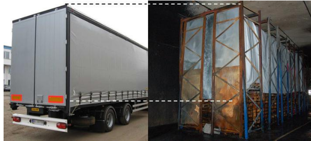
Figure 4. Real trailer and simulating mock-up [31]
